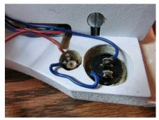
you will need to connect a wire from the center terminal (positive) of the power jack to one of the switch lugs as shown. Note carefully the polarity of the wires coming from the switch and the power jack.
